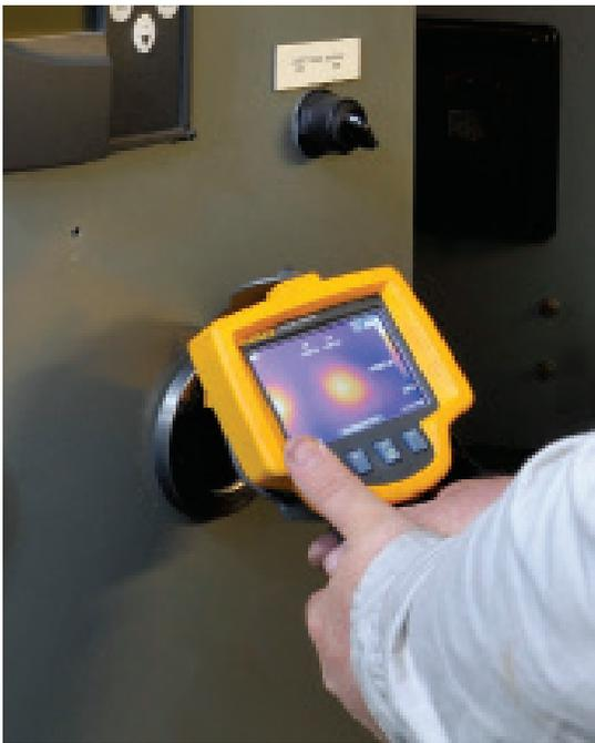
Infrared inspections use an infrared camera to detect anomalies not noticeable to the naked eye. In an electrical setting, infrared inspections identify hot spots, which can be a precursor to equipment malfunction, which leads to unplanned downtime. Heat rise in electrical equipment can be the result of:
